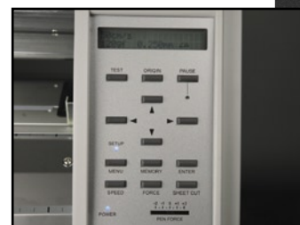
Convenient front panel makes it easy to adjust blade force, cutting speed and origin point. It also stores cutting conditions for up to eight pre-set jobs. (GX-PRO Front panel shown.)
